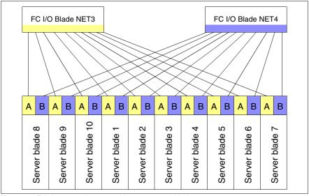
Figure 58: Fabric port assignment with 2-way server blades
